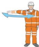
Move towards the shunter
